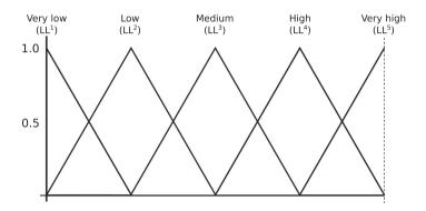
Fig. 1. Example of fuzzy partition for a continuous variable with five linguistic labels.
