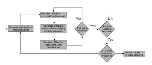
Fig. 4. General Operational scheme of the EvAEFP-Spark algorithm.
