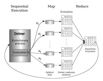
**Fig. 5.** Scheme of the evaluation procedure of the EvAEFP-Spark algorithm following a MapReduce approach.
